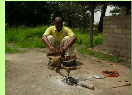
Forging using Animal Skin Bellows
